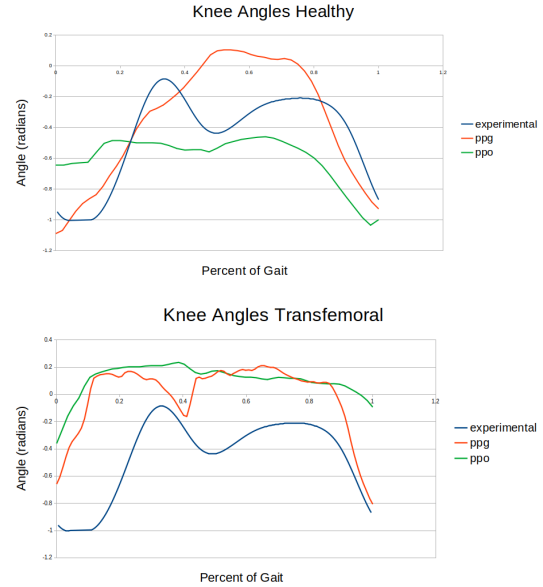
Figure 4.3: Knee angles shown for the healthy (left) and transfemoral (right) models, plotted against the experimental data
